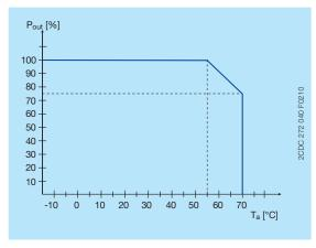
Characteristic curve of temperature at  $\boldsymbol{U}_{\text{out}}$
